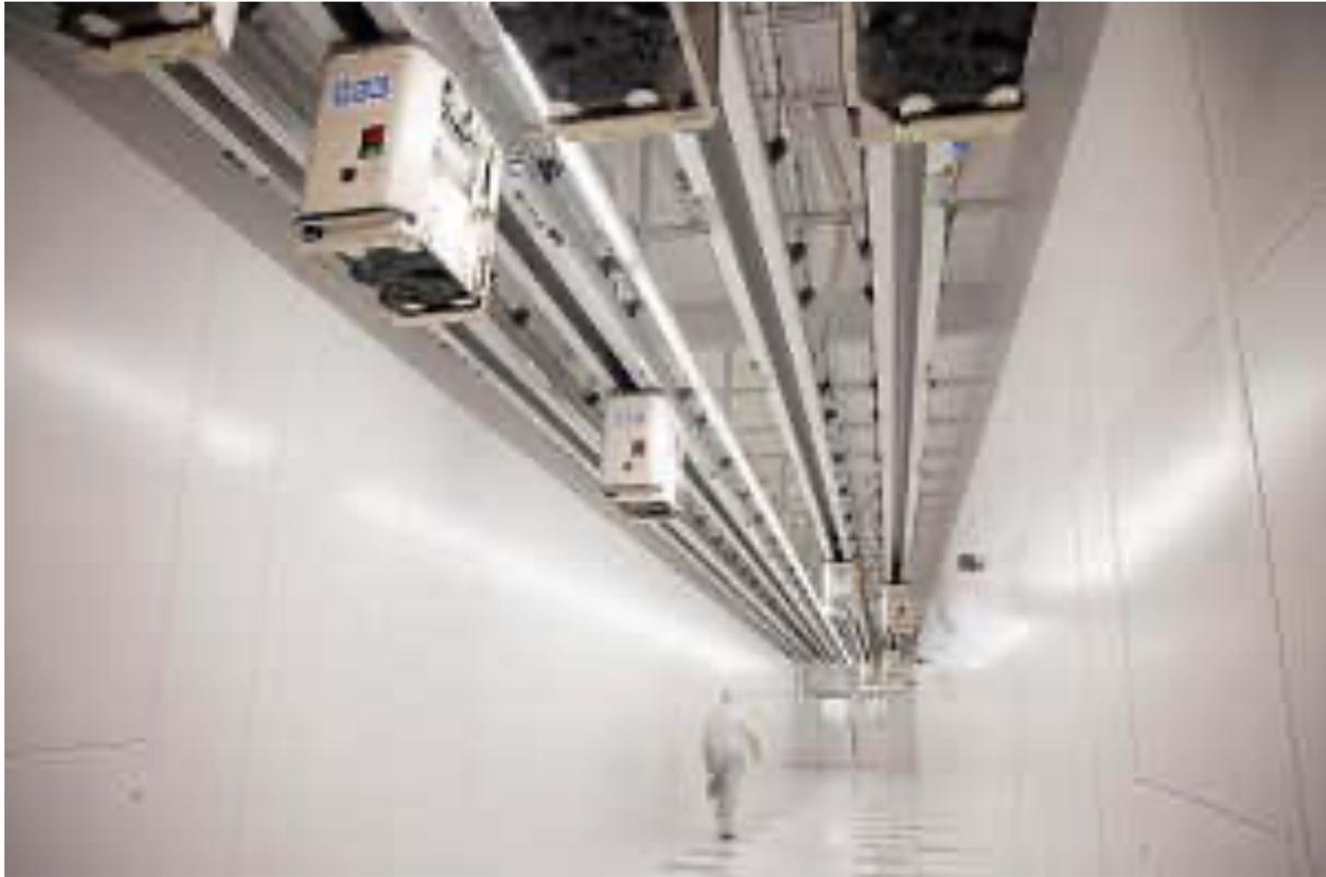
Silicon wafers being transported in clean rooms at the GlobalFoundries semiconductor plant in Germany
