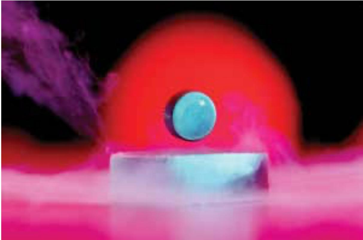
The strong magnetic fields from some superconductors can levitate objects
