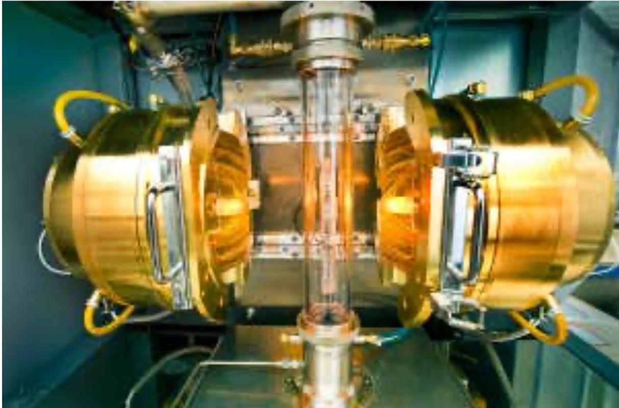
Superconducting crystals are grown in an infrared furnace at Brookhaven National Laboratory in New York state
